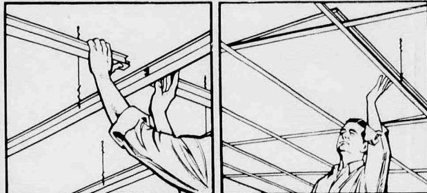
EASY STEPS TO A SUSPENDED ACOUSTICAL ceiling are illustrated here. Left, wire supports grid system, and grid snaps together. Then 2' x 4' Fiberglas panels can be dropped into place. Acoustical panels from Owens-Corning-Fiberglas.
